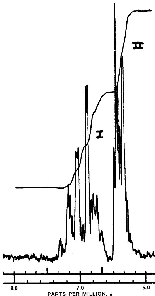
Figure 3 —NMR spectrum of resorcinol-phenol-boric acid solution. Key: I, integral for the C-2 proton of resorcinol and the five protons of phenol; and II, integral for the C-4, C-5, and C-6 protons of resorcinol.
